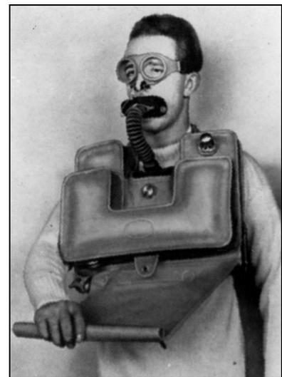
**Figure 1-10.** Original Davis Submerged Escape Apparatus.
